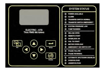
**Description**—Firetrol® FTA1250 Part Winding Starting Fire Pump Controllers can be used where the characteristics of the power source do not permit full voltage starting. The controller monitors, displays and records fire pump system information.
